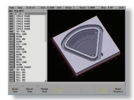
Bring a brainstorming session to life with simple features that reduce programming time. DXF file input allows the operator to import part geometry directly from a CAD file. After the DXF file has been loaded, save on MILLPWR<sup>G2</sup>'s large internal memory, USB or on your PC (via Ethernet) for easy retrieval later on.
