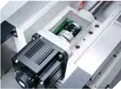
Axes motors are direct driven.
