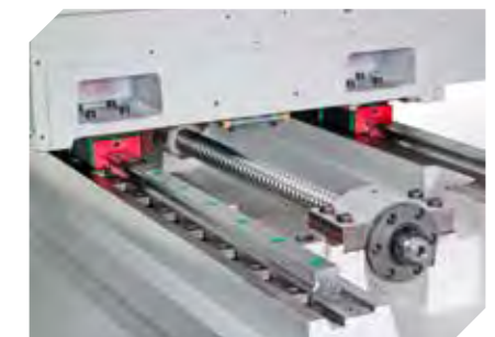
Linear Guideways suitable for fast cutting to ensure the fine cutting surface and quality for high precision requirement.
