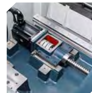
Axes motors are directly connected with ballscrews which provide high efficient movement control and lower noise features.
