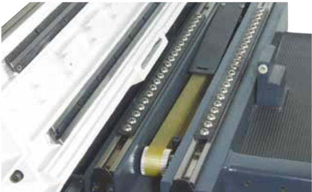
Patented steel wire timing belt transmission system (for 618m / 818m only) high precision slides way and steel balls assemble that allow lasting accuracy and smooth movement.
