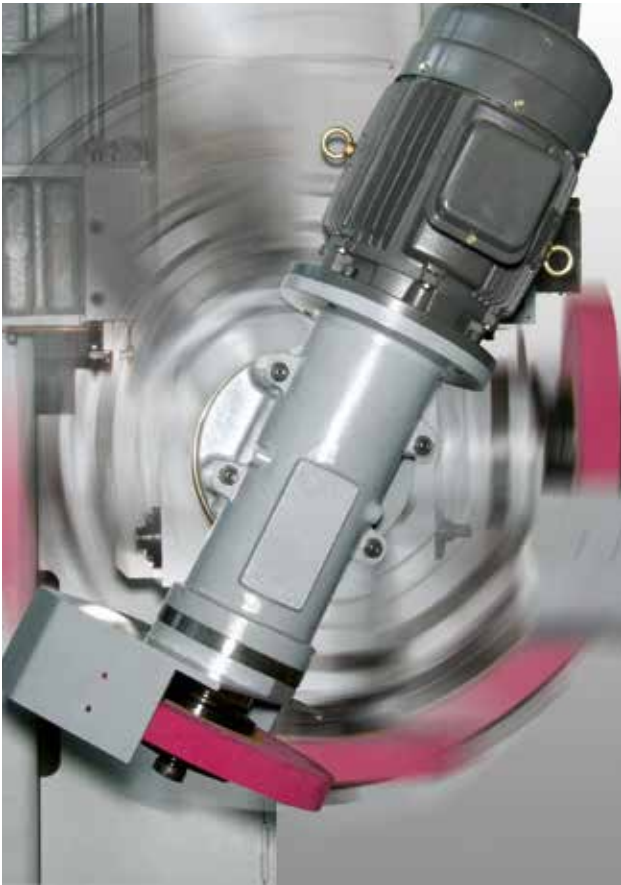
Swivel vertical spindle provides simple operation. Adjustable angle for high efficiency grinding
