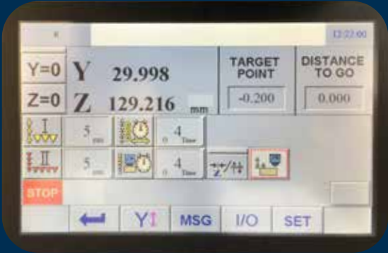
Downfeed (rough grinding, finish grinding, sparkout setting) minimum display unit: y axis 0.001Mm / z axis 0.001Mm
