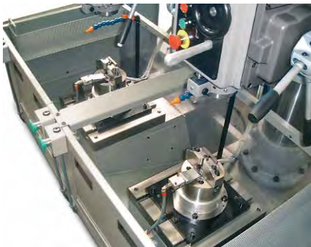
Hydraulic self-centering clamping tools for automation hinge.
