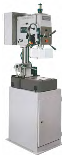
EKS-18 With lead screw system
