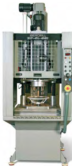
Multi-spindle headstock drilling of car handwheels, under strict technical and security standards.
