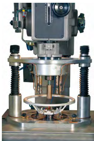
Multi-spindle headstock drilling detail of car handwheels.
